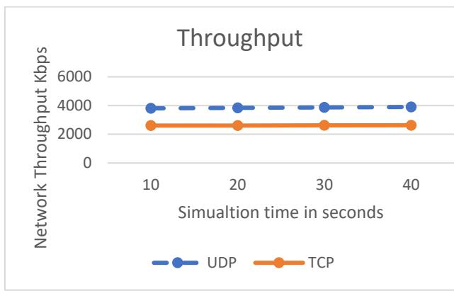
Fig. 5. The Network Throughput Of TCP Against UDP For Li-Fi Simulation
