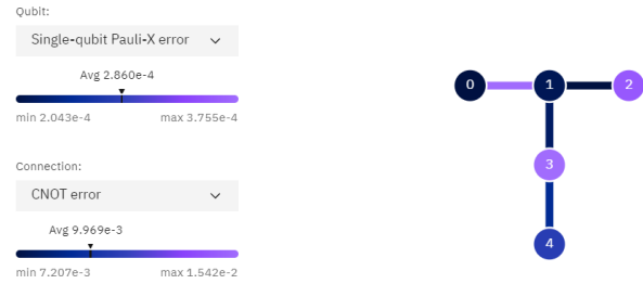
Figure 9: The qubit topology of IBM-Q Belem 5-qubit quantum system [1]
