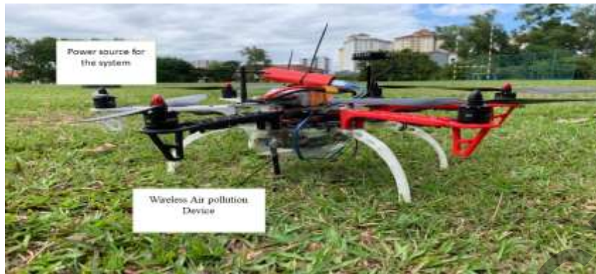
Figure 4 Integration detection station and Hexacopter drone
