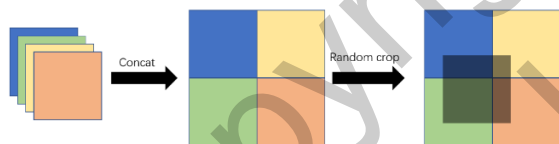
Figure 2.3.1 The process of mosaic data augmentation
